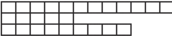
Figure 15-1: View of a jagged array
